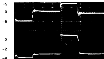
Time Base: 5 \mu Sec/Division Upper Trace: Drive Transformer Secondary Lower Trace: Power Transistor Base Voltage
